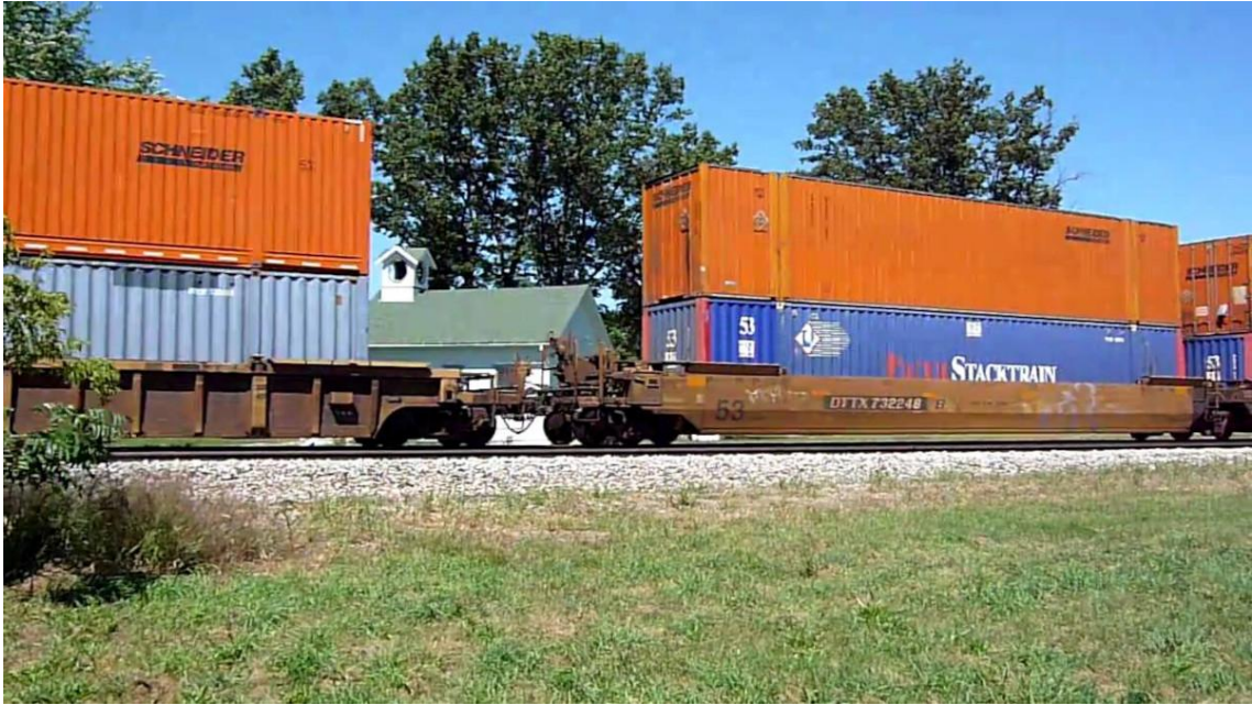
Two 53 ft double stack IM cars. Ribbed car on the left much more likely to be rideable than smooth car on the right.
