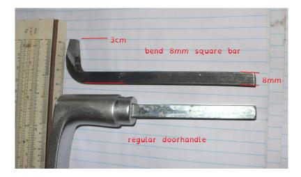
The abri, or bus-stop poster frames. But also the stand-alone rolling poster frames have a simple locking mechanism with a "key" that you can buy at a hardware store. If you are lucky, the company uses the square door handle mechanism, in some regions there is limited space so you have to make your own 8mm square bar with a bend like this one for Zeist.
